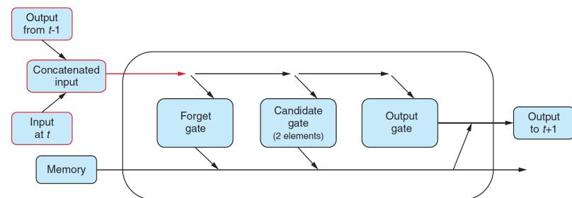
**Input:**  $[x_{[t,0]}, x_{[t,1]}, \dots, x_{[t,299]}, h_{[t-1,0]}, h_{[t-1,1]}, \dots, h_{[t-1,49]}, 1]$
